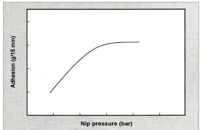
Figure 3: Effect of Nip Pressure on Adhesion of Extrusion-Coated LDPE to Porous and Non-Porous Substrates
