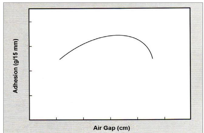
Figure 4: Effect of Air Gap on Adhesion of Extrusion-Coated LDPE to Non-Porous Substrates
