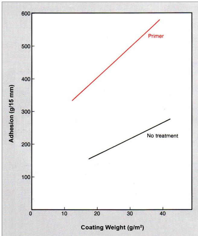
Figure 5: Typical Effect of Coating Weight on Adhesion of Extrusion-Coated LDPE to Aluminium Foil (60 m/min, 307°C)
